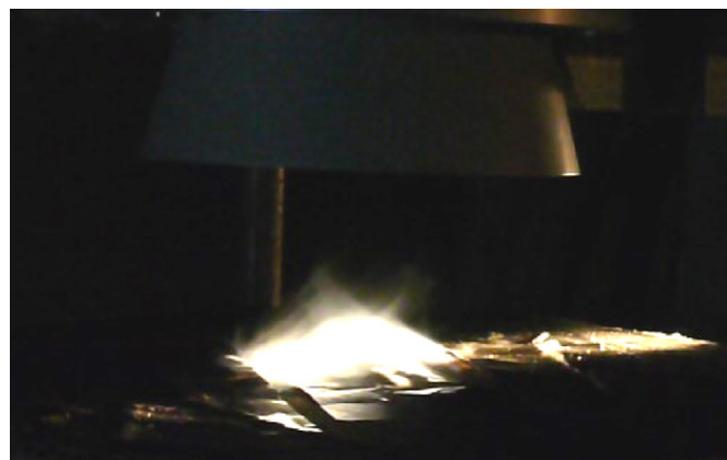
Fig. 2. The process of a gas dynamic focusing of alcohol vapors by a vortex sampler.
